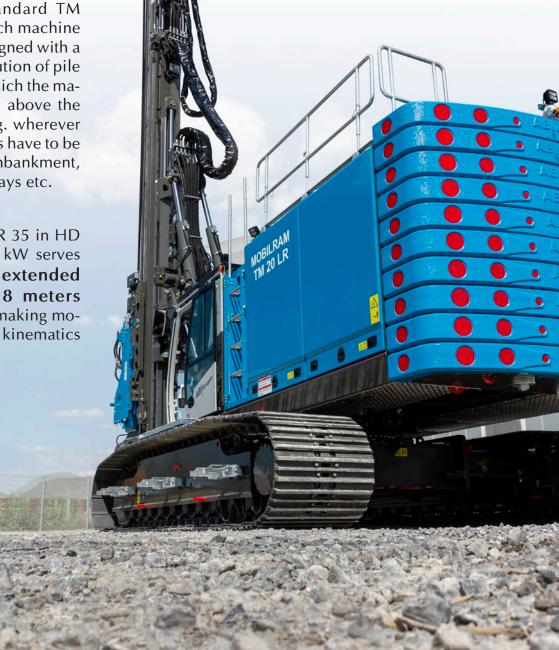
The machine complies with the EU Stage V and US EPA Tier 4 final emissions regulations. The installed C18 engine is already very efficient in itself; the diesel consumption is further reduced by utilizing the Efficiency Drive control package.
