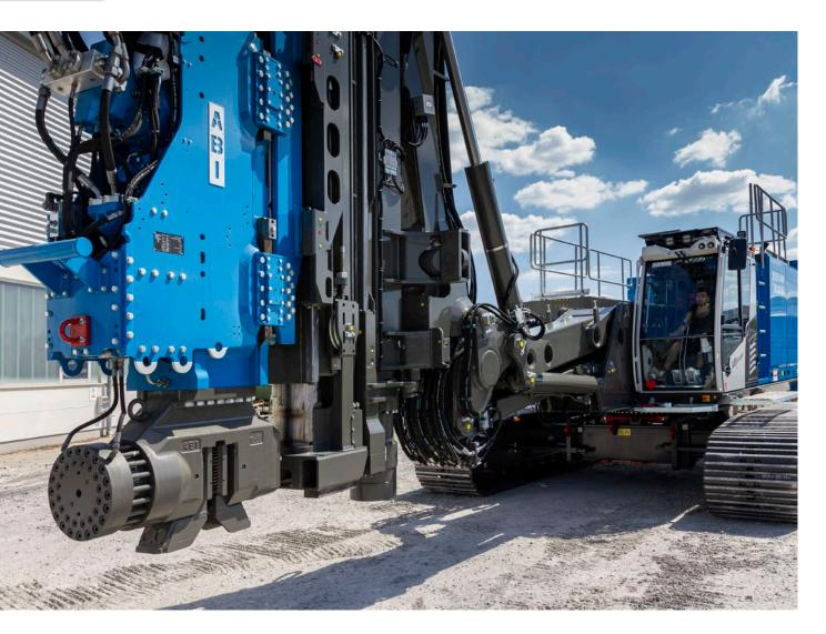
The installed engine capacity is ideal for the operation of vibrator models from MRZV 20VV with 20 kgm static moment. Via the VV technology, the static moment and the hydraulic displacement can be optimally adapted to the
