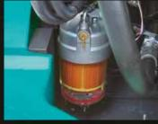
**Enlarged fuel filter** The enlarged fuel filter with built-in water separator maximizes filtering performance.
