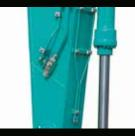
Piping for Quick Hitch A quick hitch hydraulic line, which speeds up attachment changes, is available.
